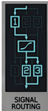
Filters' and clipper's signal routing
